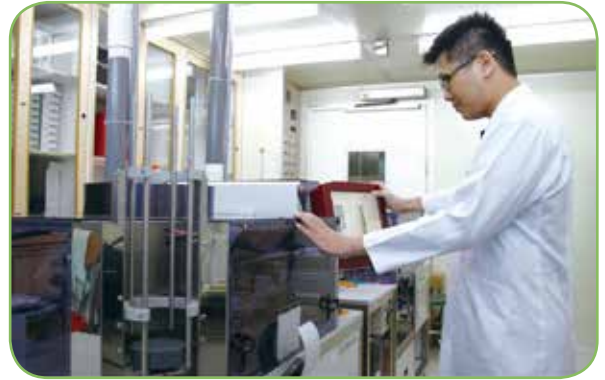
➤ Detection of substance harmful to health in tobacco products through smoking machine and gas chromatograph-mass spectrometer
