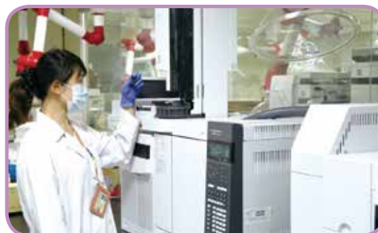
Detection of substance harmful to health in tobacco products through smoking machine and gas chromatograph-mass spectrometer
