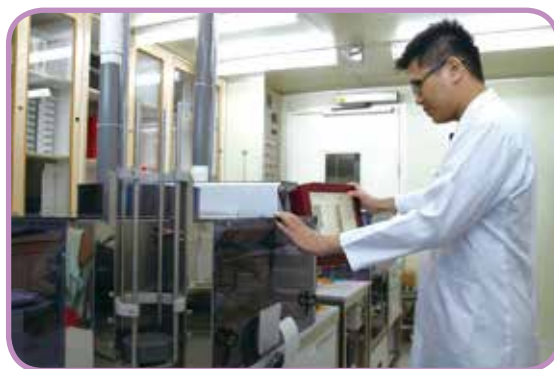
■ Detection of substance harmful to health in tobacco products through smoking machine and gas chromatograph-mass spectrometer
