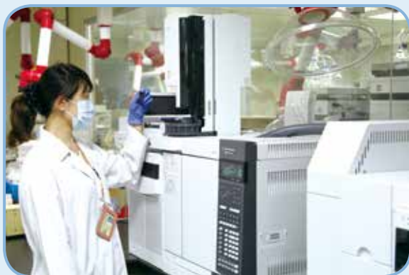
● Using a smoking machine and gas chromatography mass spectrometry (GC-MS) to detect substances that are hazardous to health
