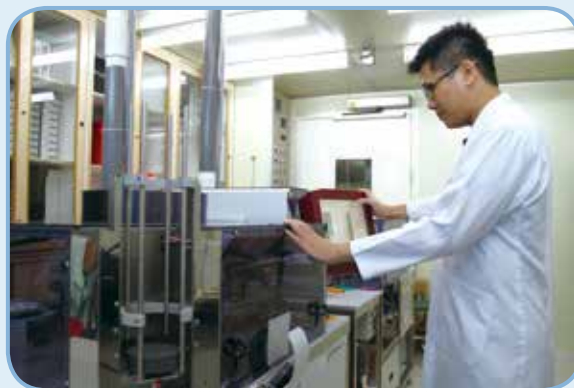
● Using a smoking machine and gas chromatography mass spectrometry (GC-MS) to detect substances that are hazardous to health
